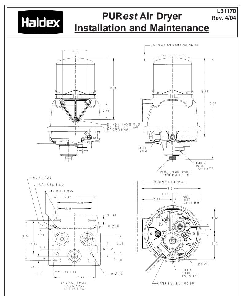
The Haldex PUR*est* is a desiccant type dryer that effectively removes moisture, oil and contaminants from the compressed air system. This reduces the risk of freezing or corrosion of the components in the air system. When compressor cut-out is reached, dry air is allowed to flow back to regenerate the desiccant bed.
