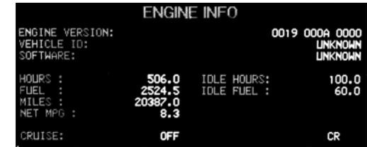
Included on this screen is data on the engine hours, fuel, miles, VIN, engine version, and idle time. These values are from the engine’s internal memory, and are accurate from the moment the engine was built, regardless of when the engine or VMS was installed. The miles value does meet the requirements as an odometer for reporting purposes when selling the vehicle.
