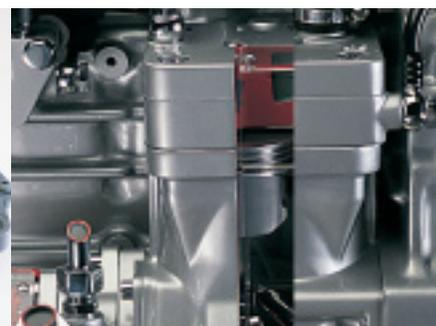
The gear-driven air compressor uses 50 percent less power, leaving more power for driving and helping to reduce fuel bills.
