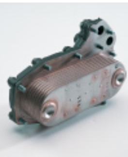
An integral engine oil cooler keeps lubricant temperatures low, promoting longer bearing and component life. The internal design reduces the risk of oil leaks.
