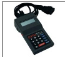
The Pro-Link handheld reader is a durable diagnostic tool for maintenance and troubleshooting. It is used in conjunction with the Multi-Protocol Cartridge and the MBE 900 data card to provide information such as a data list, limited parameters and service routines.
