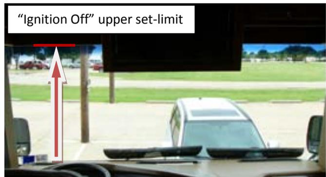
4. Turn the ignition on. Press and hold the learning key button. While holding this button, press and hold the Down switch. The motor will move in the down direction; continue holding both the button and the switch until the motor chirps and the shade stops. Once the motor chirps and the shade stops, release both buttons. The motor is now in the Set-Limit Learning Mode.
