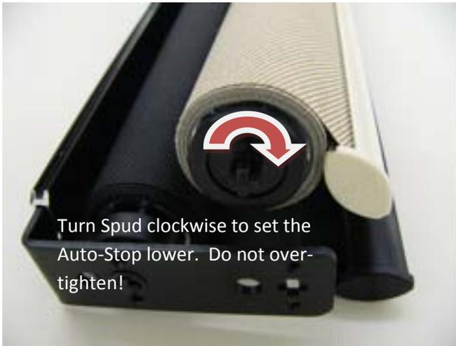
NOTE: Do not over-tighten the Auto-Stop!! Finger tight is sufficient. When reassembling shade assembly, do not compress the brackets too tightly. There should be a slight amount of clearance between the bracket and the end of the Auto-Stop and Spring. If there isn't sufficient clearance, the shade will bind.
