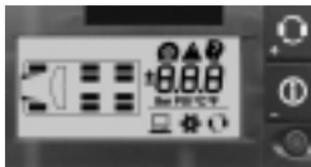
Mount the display unit and connect to power source. When power is applied to the receiver, the Full Function Display momentarily turns on all icons, beeps, and the alarm light blinks once. The unit then goes into stand-by mode waiting for data from the wheel transmitters.
