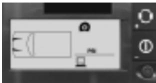
This function changes the low-pressure warning threshold for each axle.
