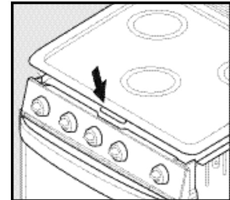
2. Slide the top on the range with the tabs of the hold down clips fitting into the slots on the back of the top.
