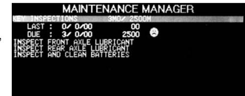
Turn the **Knob** to select a particular service group. The items in the group will be displayed, along with the date and odometer reading from the last time the service was performed, and when the service is due to be performed again. A face will show whether the item is due.
