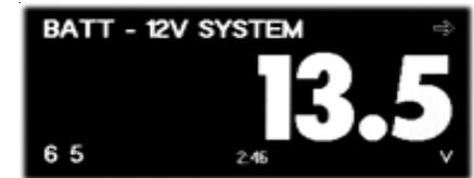
Each gauge can be displayed in two ways. The Graphic gauge shows the gauge value and two graphs. At the bottom of the screen is a simple bar graph indicating the current value. To the right is a histogram which shows how the value has fluctuated over the last minute. A flat graph indicates that the value is stable, and is not changing significantly.
