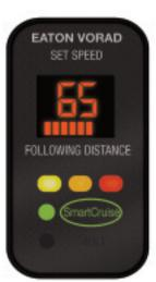
Cummins engines are compatible with all the advanced features of Eaton's VORAD accident avoidance system. These include Always Alert® road monitoring, BlindSpotter,® and SmartCruise® which automatically keeps your motorhome at a safe following distance when using cruise control.
